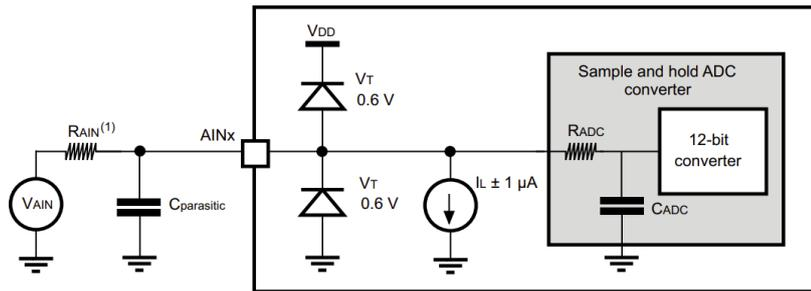
FIGURE 4.5: The schematic of ADC that compacts in STM32F303ze [37].
