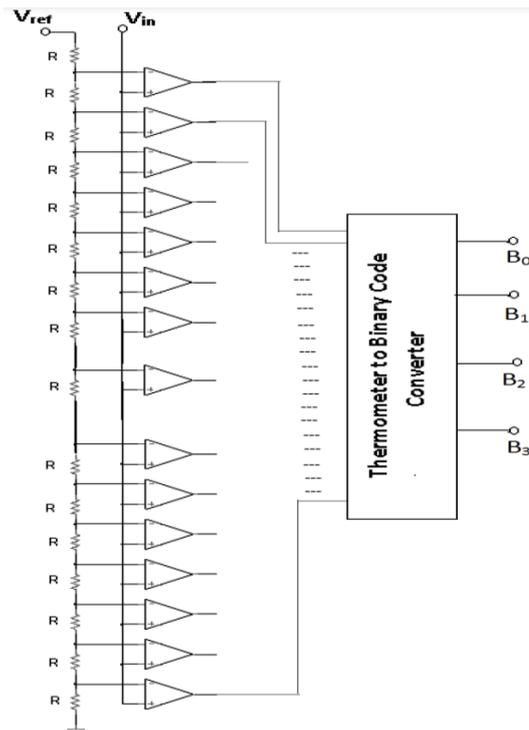
FIGURE 2.11: Architecture of 4-bit Flash ADC [24].
