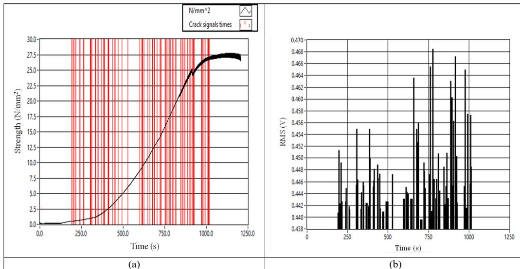
FIGURE 6.2: (a) Occurrence of the AE signals with respect to the load curve during specimen compression. (b) The AE RMS values correspond with the stress curve.
