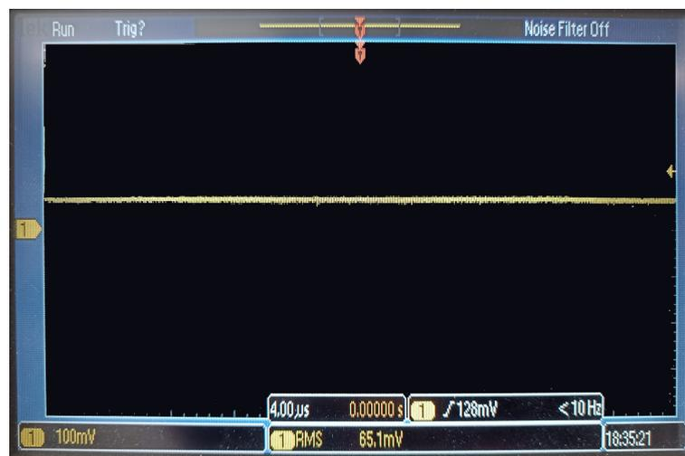
FIGURE 6.4: The offset DC signal.
