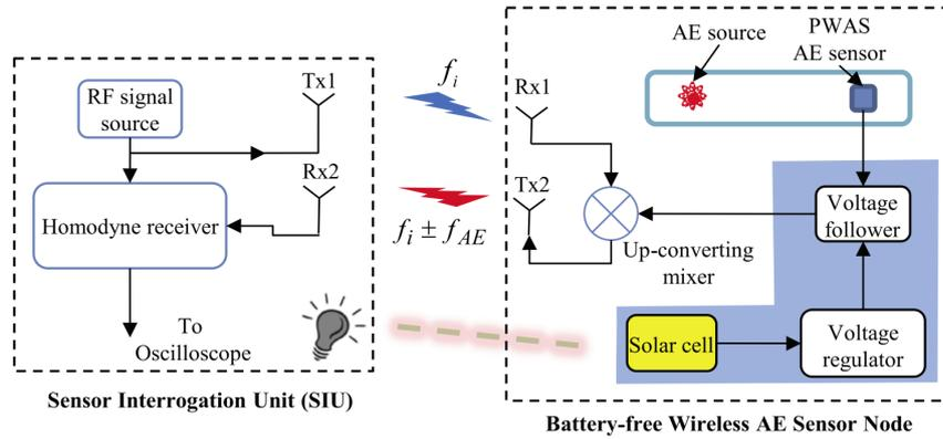
FIGURE 3.5: Wireless AE sensing system powered by solar energy harvester [32].
