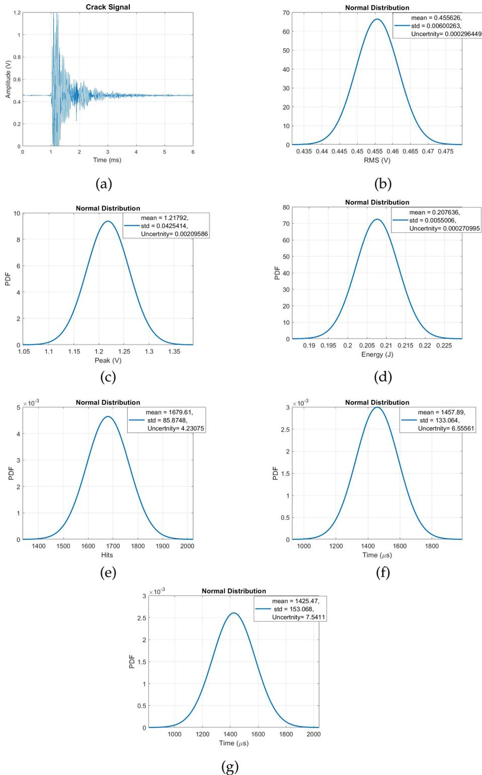
FIGURE 6.8: (a) The crack signal under study, (b) The RMS distribution, (c) The Peak distribution, (d) The Energy distribution, (e) The Hits distribution, (f) The Duration of signal distribution, (g) The Decay of signal distribution .
