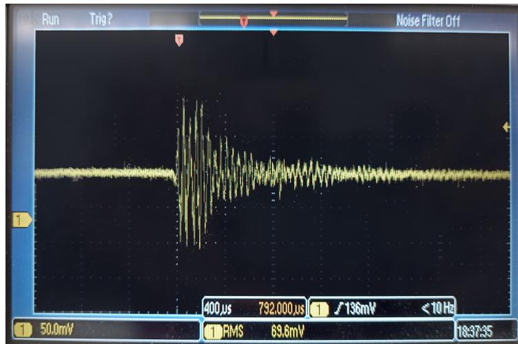
FIGURE 6.5: The AE signal with the DC offset on the input port.
