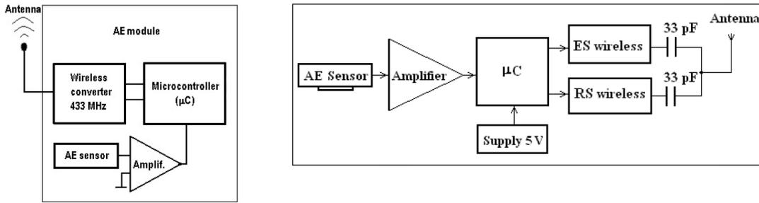
FIGURE 3.1: Block Diagram of experimental wireless module acoustic emission sensor [29].
