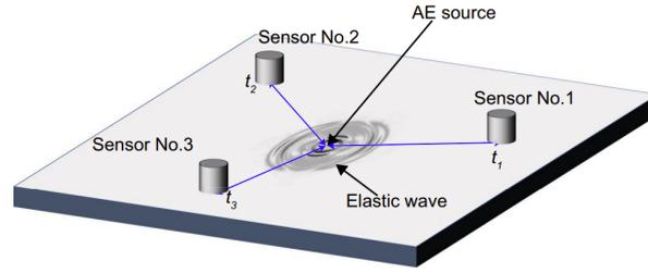
FIGURE 2.3: Schematic representation of two-dimensional localization method with three sensors [17].
