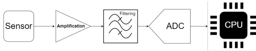
FIGURE 2.4: The main parts of AE system
