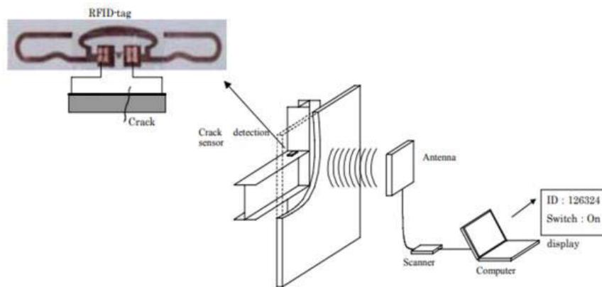
FIGURE 1.2: RFID crack detection system [6].
