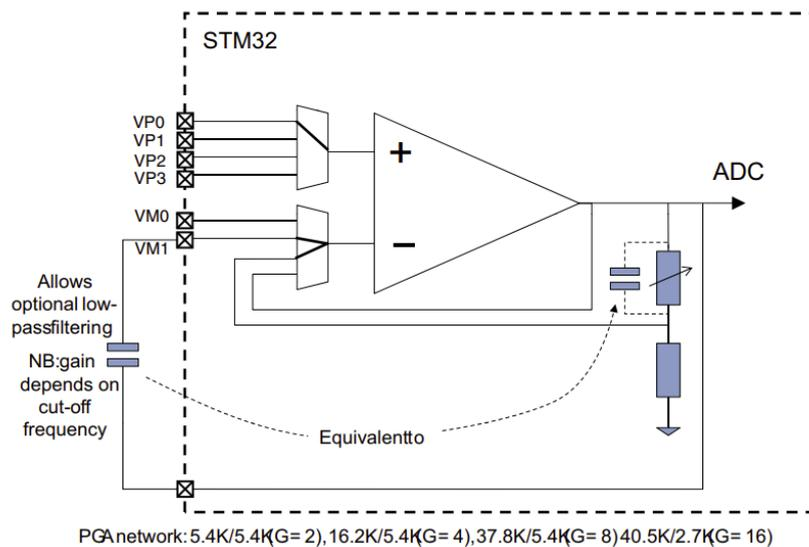
FIGURE 4.3: The schematic of a filter that compacts in STM32F303ze [37].
