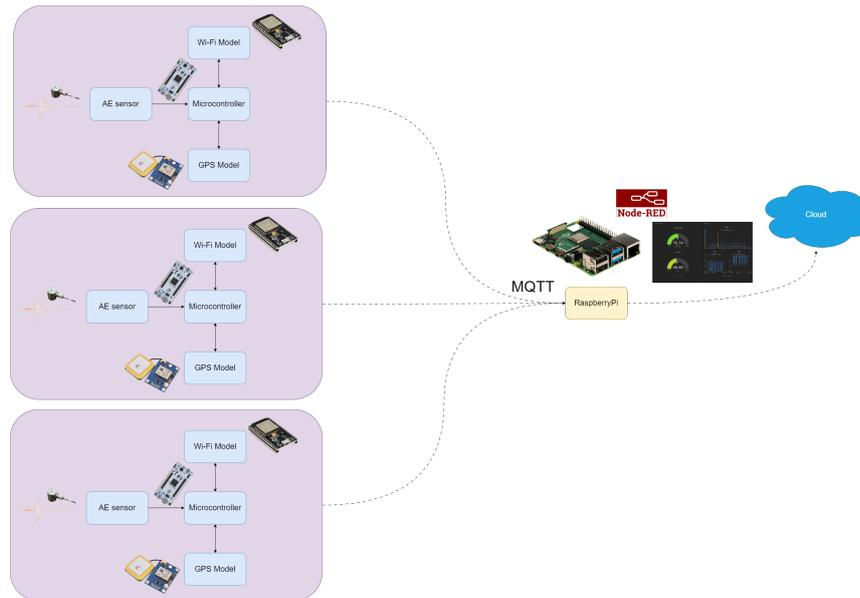
FIGURE 4.1: Conceptual diagram of the proposed system.
