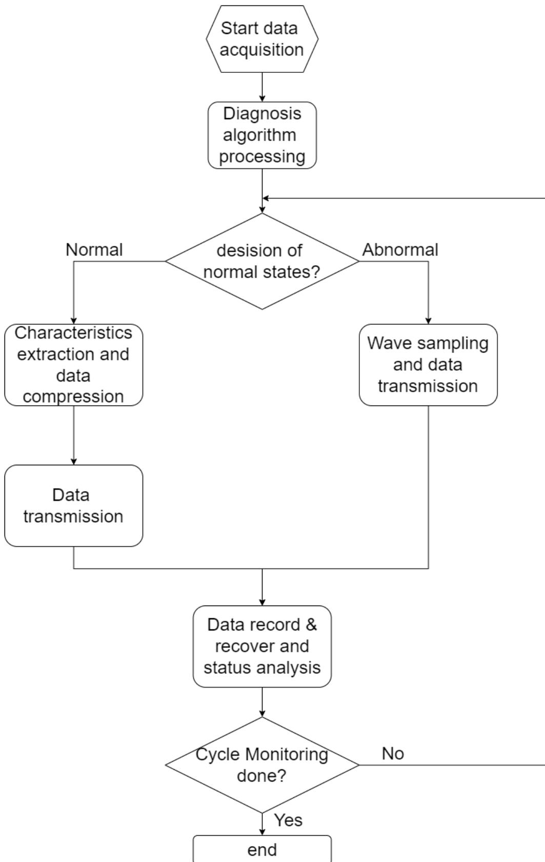
FIGURE 3.3: Operating cycle carried out by the node [30].
