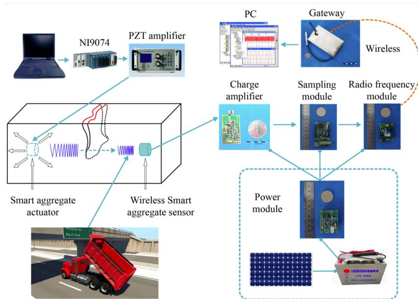
FIGURE 3.4: The architecture of proposed system by Shi Yan and et al [31].
