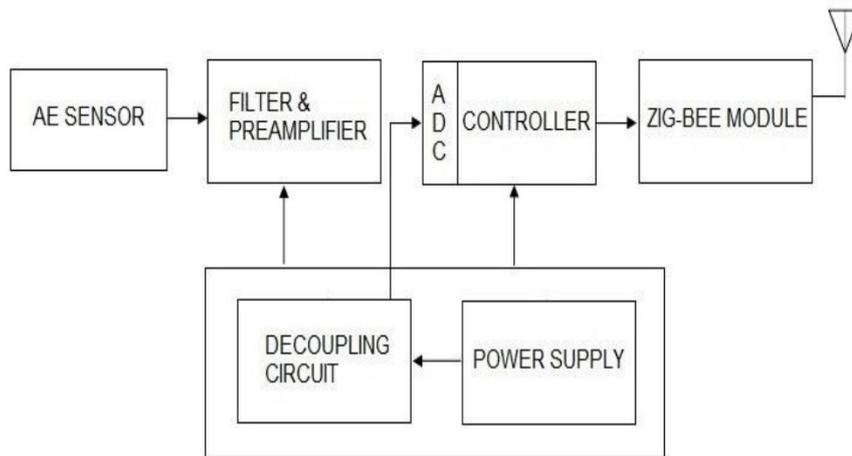
FIGURE 3.8: Block Diagram of Sensor Node [35].
