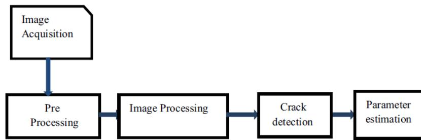
FIGURE 1.3: The architecture of image processing based crack detection [7].
