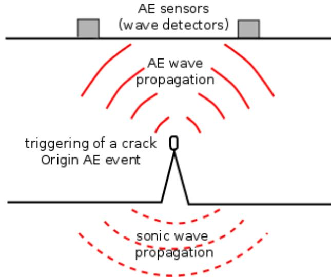
FIGURE 1.1: Principle of the acoustic emission wave detection [5].
