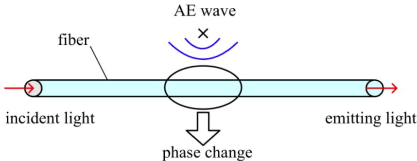
FIGURE 2.8: Optical fiber sensing principle [21].
