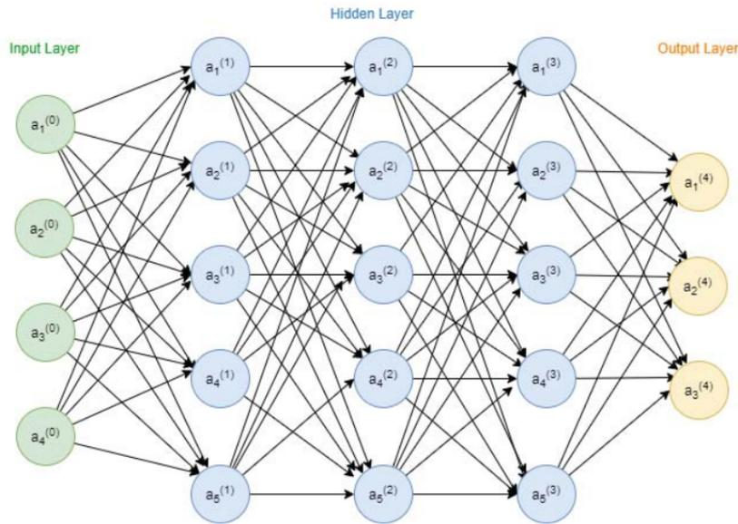
FIGURE 1.4: The architecture of the neural network [1].
