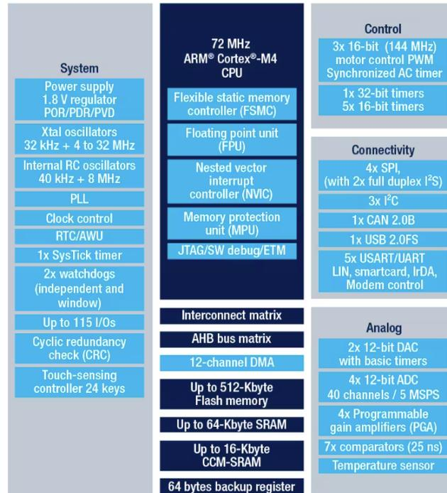
FIGURE 4.4: Circuit Diagram of STM32F303ze [37].
