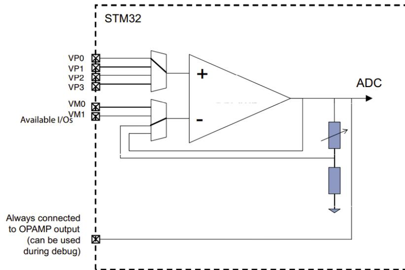
FIGURE 4.2: The schematic of an amplifier that compacts in STM32F303ze [37].
