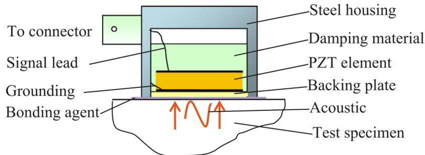
FIGURE 2.5: Cross-section of a typical commercial AE sensor [18].
