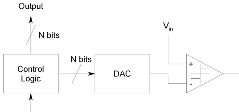
FIGURE 2.10: A schematic representation of a successive approximation ADC [23].
