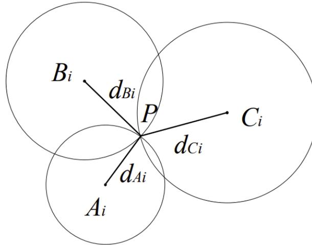
FIGURE 2.2: The diagram of trilateration positioning calculation [16].
