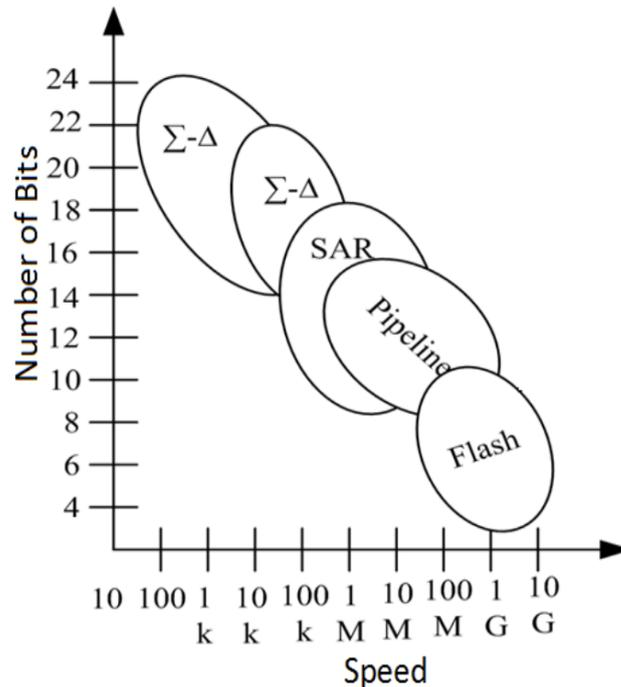
FIGURE 2.14: Comparison of various ADC architectures [24].
