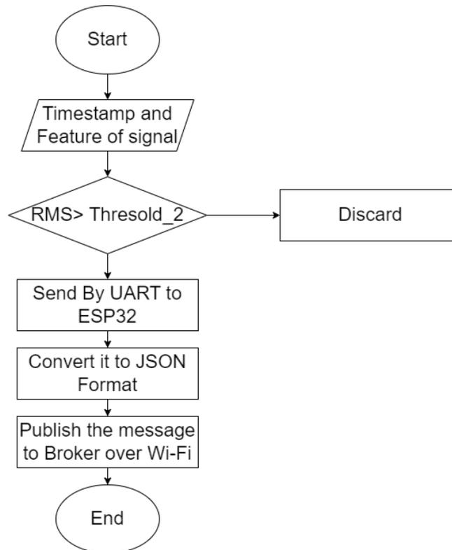
FIGURE 5.3: Flowchart of Communication Algorithm.
