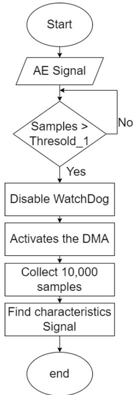
FIGURE 5.1: Flowchart of the detection AE crack algorithm.
