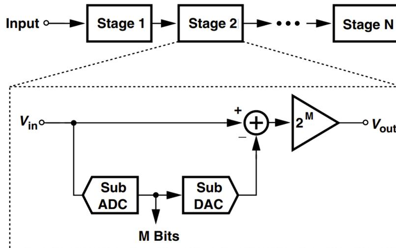
FIGURE 2.13: Pipelined ADC architecture [26].
