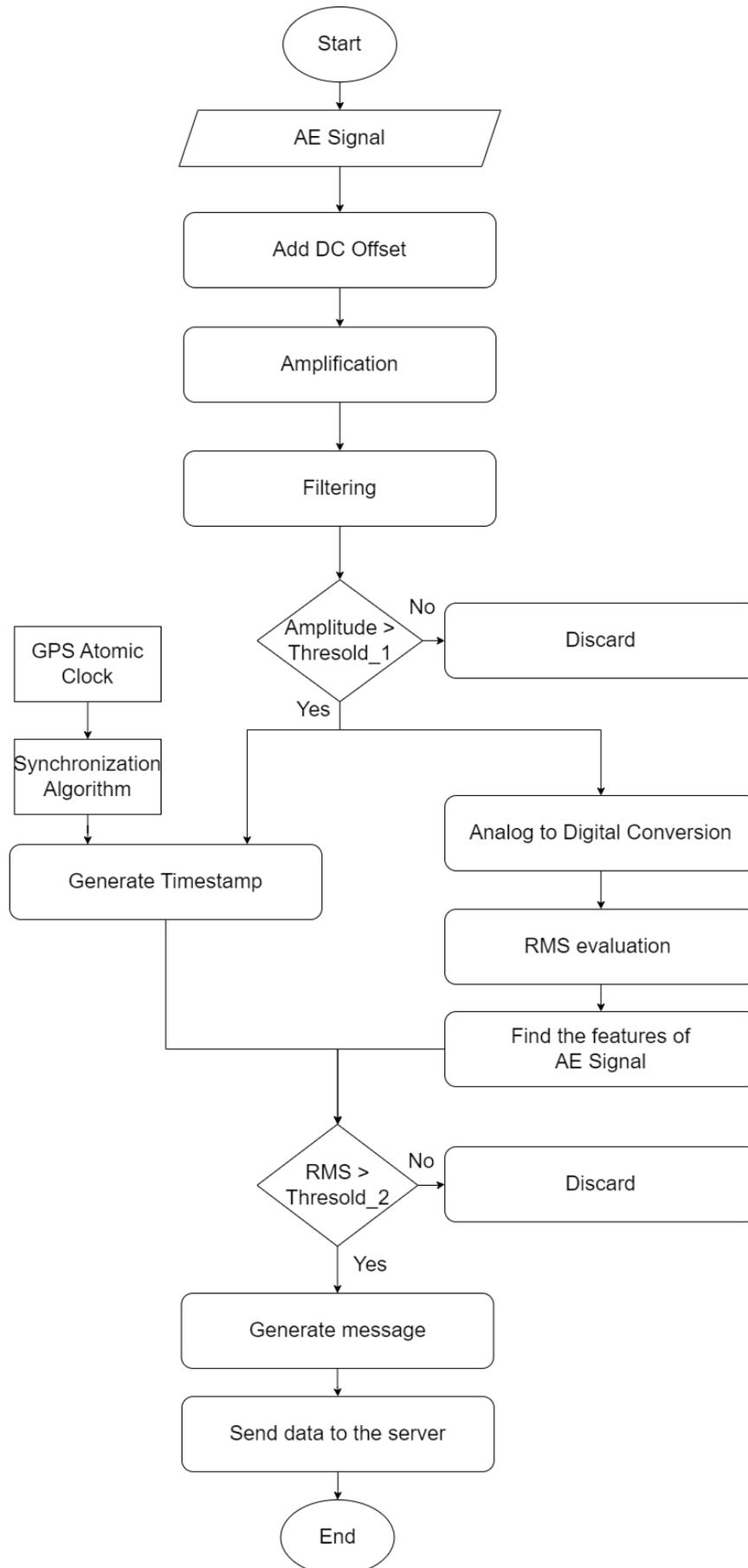
FIGURE 4.9: Flowchart of the proposed architecture.
