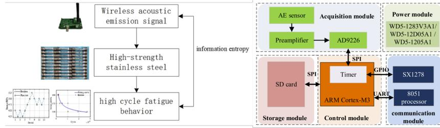
FIGURE 3.7: Hardware and implementation of the system [34].
