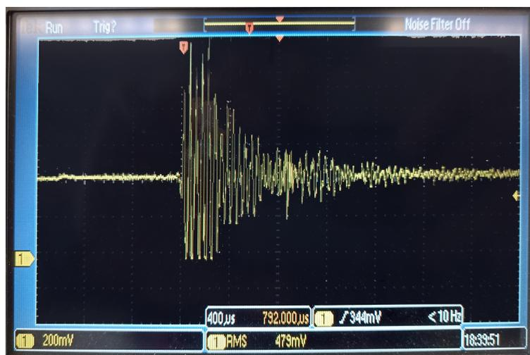
FIGURE 6.6: The AE signal with the DC offset on the input port.
