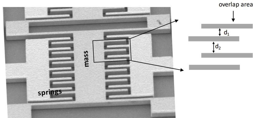
FIGURE 2.6: Capacitive MEMS AE sensor [20].
