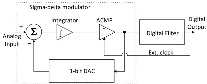
FIGURE 2.12: The schematic shows the basic building blocks of delta-sigma ADC [25].
